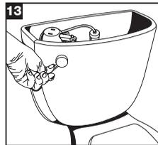
13. Flush toilet to ensure new Watts Fill Valve is installed and operating correctly. Check to see if any part of Fill Valve rubs on tank or interferes with operation of Flapper. Adjust as necessary.
