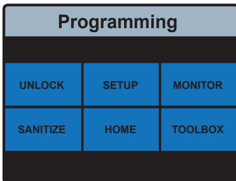
3. On the Programming Menu, touch the **UNLOCK** icon. The Unlock function screen will appear and you will be prompted to enter the passcode:
