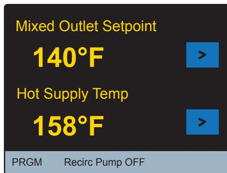
3. If the “Hot Supply Temp” is BELOW the “Mixed Outlet Setpoint”
