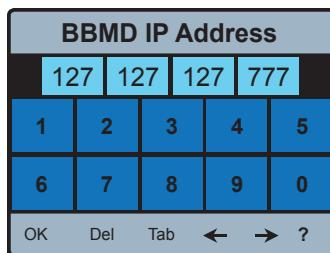
Use the **Tab** icon to move between the four groups of three numbers, use the **← →** to move around in each group of 3 numbers, and use the **Del** to delete the numbers entered in the field to allow entering a new number.
