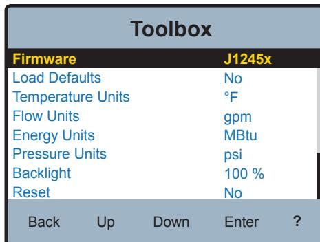
The Toolbox Function allows access to the following fields:
