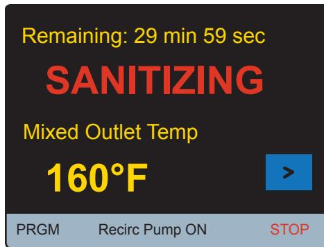
9. After Sanitization Mode has completed (user selected run time has elapsed), the IntelliStation will go into a Cool Down Mode to return to the Mixed Outlet temperature prior to sanitizing.
