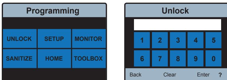
To unlock the control select the **UNLOCK** icon from within the “Programming” menu.
