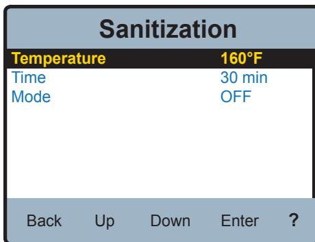
3. Select the Sanitization temperature first by highlighting the TEMPERATURE function on the Sanitization menu and then touching **Enter**.
