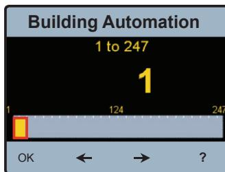
To adjust the “Modbus Address” either press anywhere on the slider bar and/or use the arrow keys and then select **OK** to save the setting and return to the “Building Automation” menu. The “ModBus Baud Rate” and “Modbus Parity” are adjusted in a similar fashion.
