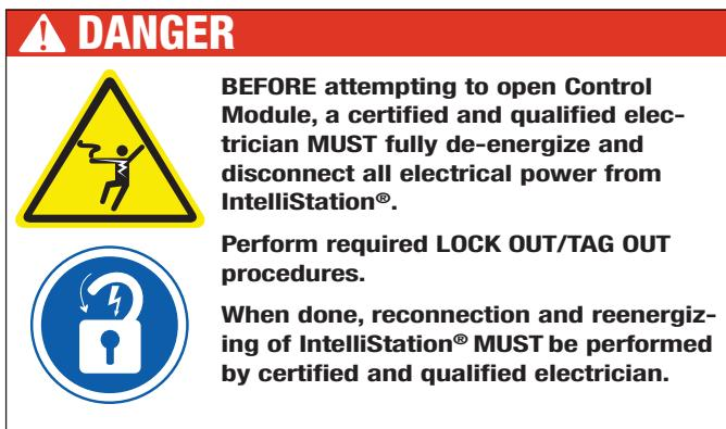
3. Disconnect all power and fully de-energize IntelliStation® BEFORE opening the control module. Open the Control Module and locate the non-functioning sensor.
