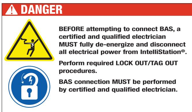
1. After completely de-energizing and disconnecting all power from IntelliStation® and performing required LOCK OUT/TAG OUT, carefully open the IntelliStation control module by releasing latches to reveal BACnet® and Modbus® hook up terminals.
