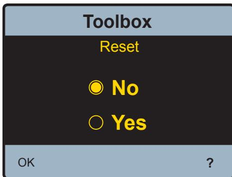
7. Press the **OK** and then **OK** and the control will reset and begin a start up sequence.
