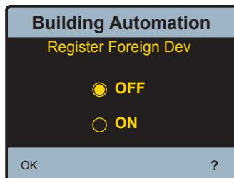
To toggle from “OFF” to “ON” press on the **OFF** icon next to the “ON” setting to change the **OFF** icon to **ON** indicating that this state is what is selected. Press **OK** to save this setting and return to the “Building Automation” menu shown below with “Register Foreign Dev” set to “ON”. Note the additional setting available with the “Register Foreign Dev” set to “ON.”
