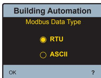
To toggle from “RTU” to “ASCII” press on the  icon next to the “ASCII” setting to change the  icon to  indicating that this state is what is selected. Press **OK** to save this setting and return to the “Building Automation” menu.
