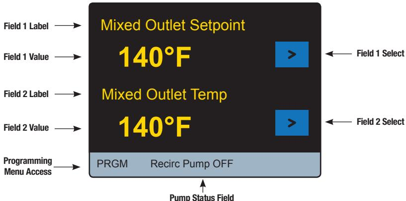
As shown in the screen shot above, there are two fields viewable within the “Home” screen. For instance, the Label (item) and Value for Field 1 and Field 2 shown in the Home screen view above are:
