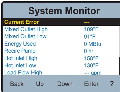
**The Monitor Function allows access to the following fields:**
