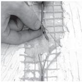
**Step 3.12.** Slide the solder tube over one of the heating wires.
