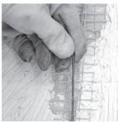
**Step 3.5.** Use a glove or other protective cloth to pull off the loosened jacket slug. **Do not touch** the hot jacket slug with bare fingers. The slug will be very hot and will burn!
