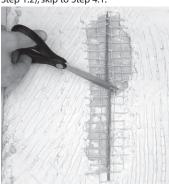
Step 3.1. Cut out the damaged wire location, creating two ends or leads. If the cable being repaired is not the jacketed heating cable, skip to Step 3.6.
