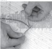
Step 4.8. Use the small screwdriver, paper clip, fingernail, or similar instrument to pry between the braid and make an opening through which to pull the heating wires. Pull each wire through the braid.
