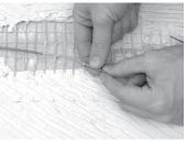
Step 4.6. Loosen the braid by pushing back on the braid about 1/2", causing the ends of the heating wires to be exposed. **Note:** Some of our heating cables do not have a braided ground shield. These cables will have a ground drain wire and a foil wrap. Simply remove the foil and proceed to Step 4.10.
