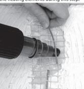
**Step 3.4.** With either type of jacket, if it doesn't easily pull off you may need to use your heat gun to gently warm the slug, which should soften and loosen it for you. Use the heat gun (set to about 500°F) and move the gun back and forth under the jacket slug for about 3 or 4 seconds, or until it can be easily removed.
