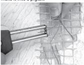
**Step 3.10.** Use the thermal wire strippers to carefully strip off exactly 1/2" of the insulation from the heating wires. Count the little heating elements to make sure none were cut off and thereby cause a hot spot or possible failure. A fiber strand may also be found among the heating elements. There is no need to separate or remove this fiber strand.
