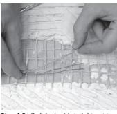
**Step 4.9.** Pull the braid straight out to make it into a pigtail.
