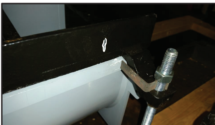
The Clip On 12" DI Frame Engages The Channel Against The Top Lip
