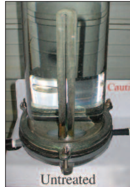
Scale Build-Up (In untreated water).
