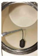
Pre Installed Float Switch
