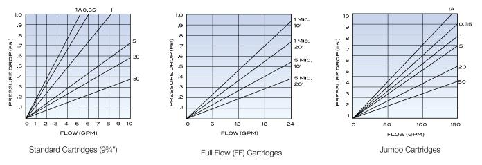
Note: Pressure drop data shown above include filter housing and cartridge.
