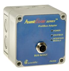
PA500 Profibus Gateway Adapter connects up to 30 Modbus Communications Modules to a Profibus DP (V0 or V1) network with M12 connector. Full-featured measurement, calibration, configuration and diagnostics. 24 VDC power.
