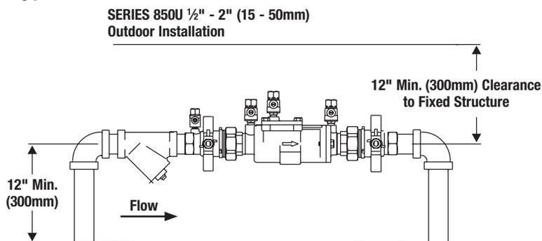
\*\*Metric Dimensions are nominal pipe diameter. This product is produced with NPT threaded end connections.
