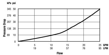
Flow curves are for reference. Actual flows may vary depending on system temperatures and/or pressures. \*\*Flow curve with integral inlet check valves and filters
