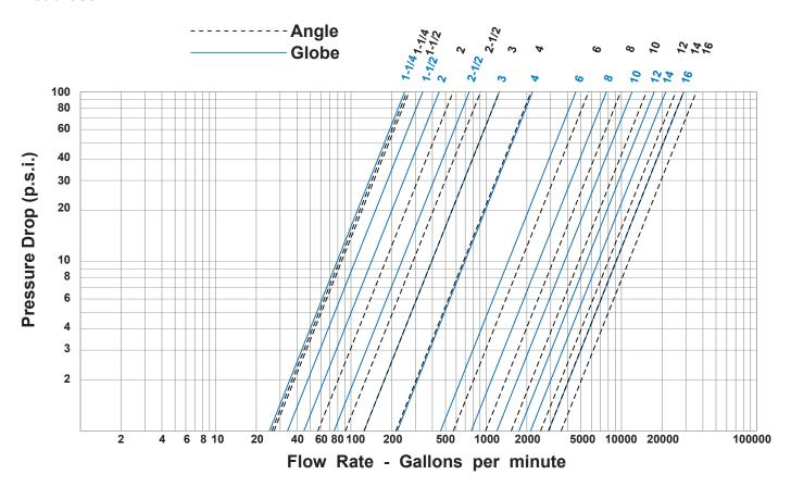
The  $C_{\nu}$  Factor of a value is the flow rate in US GPM at 60° F that will cause a 1 psi drop in pressure. The factors stated are based upon a fully open valve.
