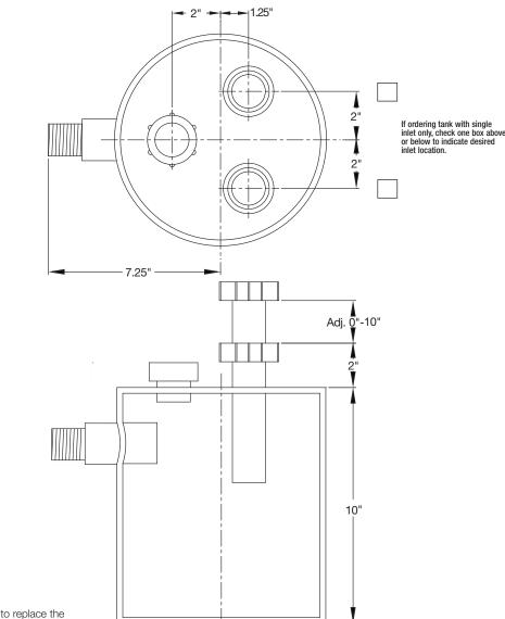
Note: Tanks are made to  $\pm 0.25$  in. tolerance.
