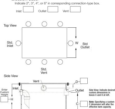
Tank Extension If required tank height exceeds standard height (H) for a buried tank, an extension may be required. Please check extension option box above. Extension height will be verified by
