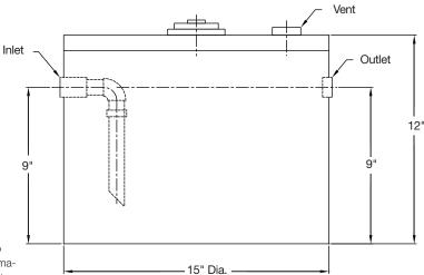
Note: Tanks are made to ±0.25 in. tolerance.
