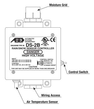
PM-2B provides integrated air and moisture detection within a rainproof and ice-resistant enclosure.
