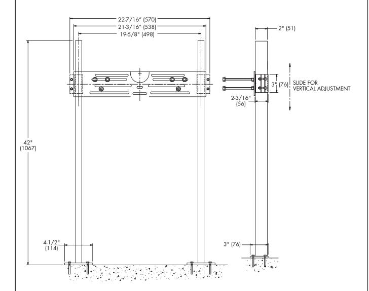
Note: Anchor legs to concrete floor with minimum 1/2" (13) anchor bolts (by others).
