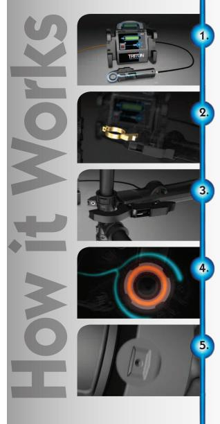
The Control Unit converts standard 110/120 VAC electrical current to DC electrical current, then generates a radio frequency (RF) signal.
