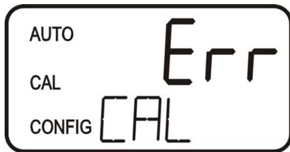
To recalibrate press the MODE key and start the calibration sequence again. To restore the factory calibration, push and hold the  $\blacktriangleleft$  button. Now push and release the  $\blacktriangleright$  then release the  $\blacktriangleleft$  button. See section [6.1 Restoring Factory Settings](#)
