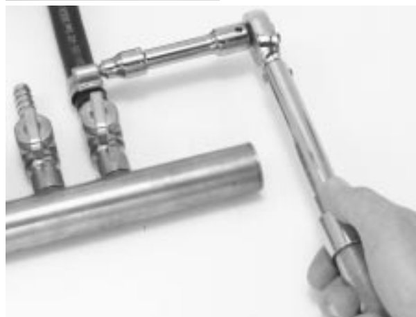
Tighten the clamp using an in/lb torque wrench.
