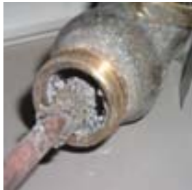
This temperature and pressure relief valve has become clogged with the accumulation of hard scale, which can lead to potentially dangerous conditions.
