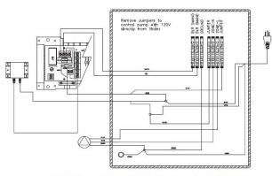
Type 3 Condensing Boiler Panel Schematic
