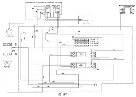
HydroNex Source Select panel Type II Schematic.
