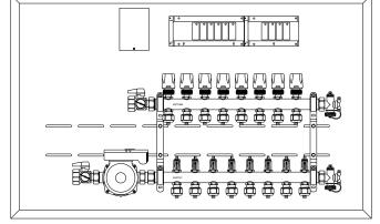
Pumped Manifold Station less Actuators
