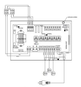
HydroNex Direct 3 zone panel Schematic.
