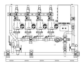
HydroNex DMix Hybrid 4 zone panel. DMix Hybrid series are available from 2 to 4 zones.
