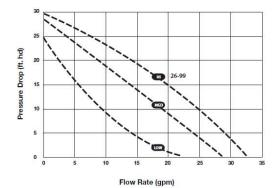
Watts Radiant (Grundfos) Circulators
