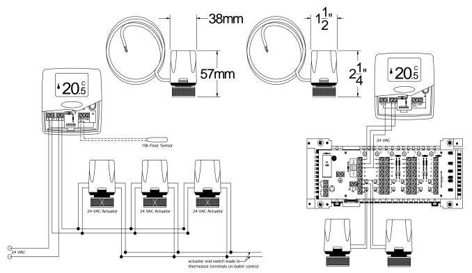
Typical Wiring of 4-Wire Actuator with End Switch
