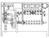
HydroNex Zone Pump Mix with actuators.
