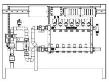
HydroNex Zone Pump with actuators.
