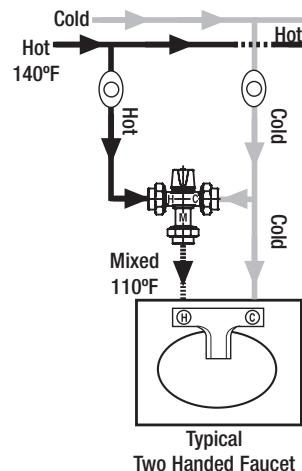
Common applications are sinks and whirlpool tubs; hence the temperature variance or control is not as tight ( $\pm 7^{\circ}\text{F}$ ) as required for a shower application.
