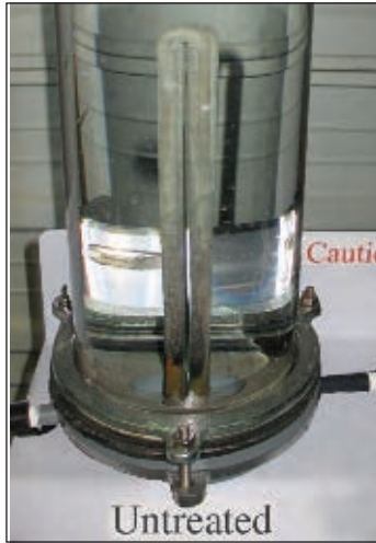
Untreated Scale Build-Up (In untreated water).
