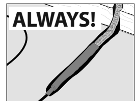
ALWAYS completely embed the factory splice and all heating wire in mortar. NEVER bend the splice or place any part of it in the wall or through the floor.
