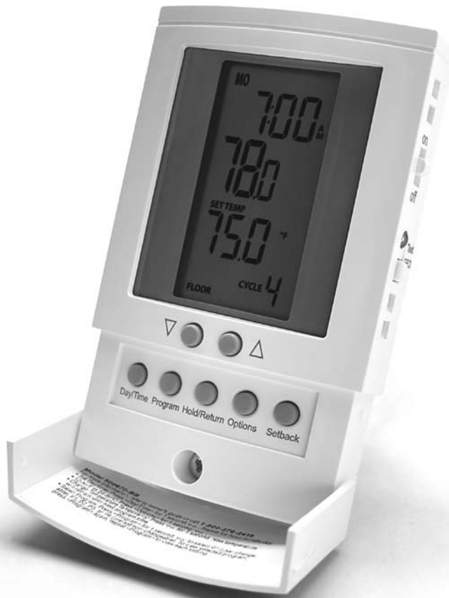
The programmable SunStat™ with built-in timer eliminates the need for a separate programmable timer. Built-in clock displays time of day and day of week, a programmable temperature set-back on a timed schedule, on/off control, manual override, and built-in GFCI. Temperatures are displayed in either °F or °C. A hinged access panel opens to reveal the programming controls. A 15-ft. sensor wire and complete instructions are included with the control.
