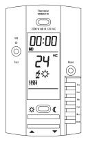
Adjust the setpoint temperature until heating indicator (()()()) appears on display. Press on TEST button. The test is conclusive if the warning light (GFI) on the thermostat is ON and power to the load is cut-off. If these events do not occur, check the installation. Press on RESET button to reset the GFCI.
