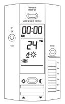
The message LO or HI will appear on the display if the temperature sensor is defective or the temperature is below 0°C (32°F) or higher than 60°C (140°F). Also, the heating indicator will be present on display and the relay will be closed (current going in the load).
