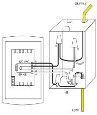
Push the excess wire back into the electrical box to prevent interference with the thermostat. Secure the thermostat using two (2) 6-32 screws. Once the thermostat is properly installed, return power to heating system.
