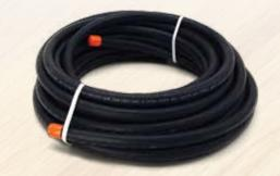
Onix is an EPDM-based, aramid fiber reinforced tube with an aluminum oxygen barrier. Its unmatched flexibility and durability make Onix the best tubing for underfloor radiant, cold weather installations, and snow melt.
