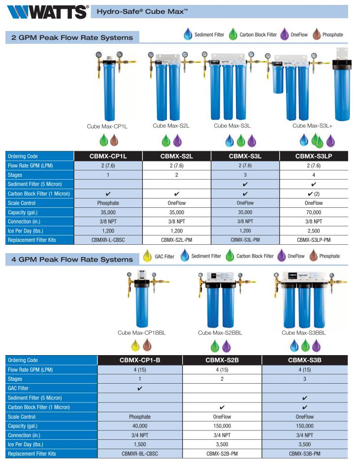
Note: All Cube Max replacement filter packages are also available with phosphate scale control as well. Filter changeout interval should be one year for OneFlow, and six months for phosphate filters. The gallon capacity claims are for dechlorination. Peak service flow rate is for intermittent use only and is not to be interpreted as continuous service flow rate capacity. See System Feedwater Requirements and OneFlow Application Practices on page 16.
